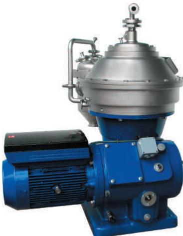
BTPX 305 solids-ejecting disc stack centrifuge
